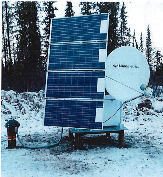
Figure 4. Photo of the new seismic station NBC1, showing the satellite dish, solar panels to power the system, and electronics – all built on a platform, and the borehole seismometer (left).
