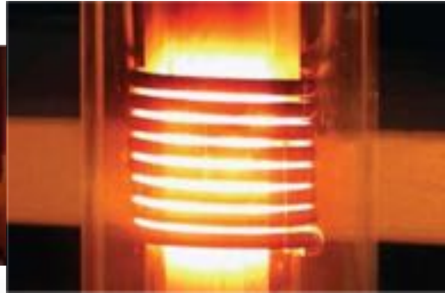
Electric Induction Furnace
